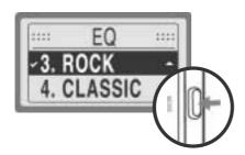
③ Press the FF/REW button to move to the desired equalizer mode and press the PLAY/STOP button to select. Press the MODE button to exit the MENU.
