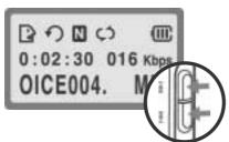
② Press and hold the FF/REW button until the desired time, the RipFlash Trio will start playback from that point.(SEEK Function)
