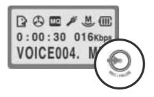
4 Press the MODE button to exit the menu and make sure the setting(VOR time) is on during recording.
