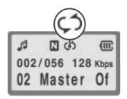
④ Press the MODE button to exit the menu. The REPEAT icon on the LCD should be lit.
