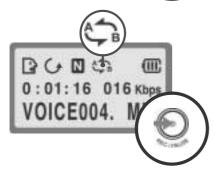
③ Press the REC button once again to set the end point(the ending of a section). The specific section you selected will be played repeatedly.
