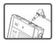
② Connect the external microphone to external jack of the RipFlash Trio using earphone connector.
