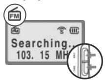
① In FM RADIO MODE, press the FF/REW button to select a channel. Press the FF/REW button two seconds (or longer). The frequency will go up/down and will seek channels automatically (Auto-seeking function).
