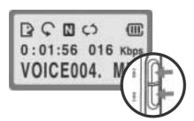
① During playback in the Stop mode, press the FF/REW button to navigate to the desired file.
