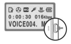
③ In the STOP state of VOICE MODE(or AUDIO MODE), press the REC button to start recording. To pause recording, press the REC/PAUSE button. To stop recording, press the PLAY/STOP button.
